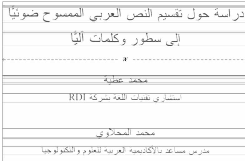
Figure (3.4): Sample text rectangle bitmap after initial lines decomposition.
