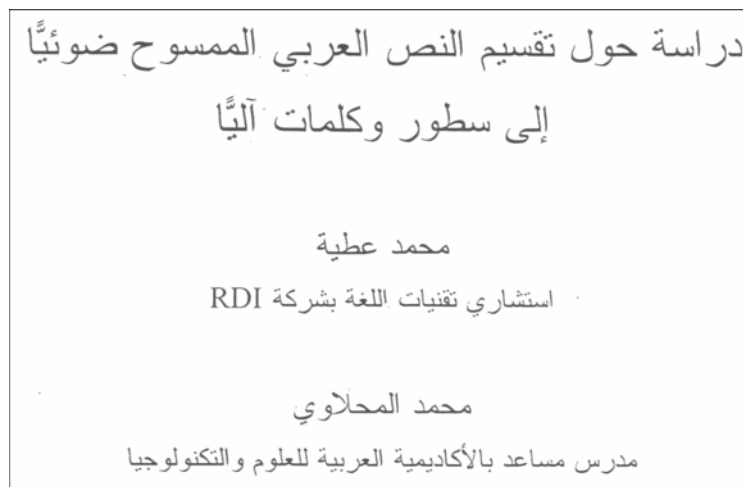
Figure (3.1): Sample Arabic text rectangle bitmap; Laser-printed, photocopied once, and scanned at 300 dpi & 256 gray shades.
